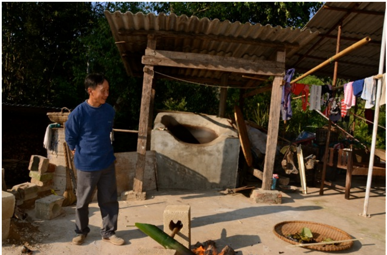
'Eggplant' stands in his yard. In the background is a tea fryer which must be covered from the sun to ensure that withered leaves that are being fried are not affected by the direct sun rays. It is for such a reason that frying is only done at certain points of the day when the sun doesn't hit the fryer.
